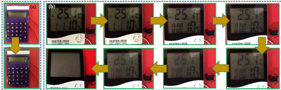
Figure 3.3.6 (a) powering up a commercial calculator using the hybrid device with charging a commercial capacitor (b) powering up of a commercial hygrometer for a period of 30 seconds by charging a commercial capacitor
