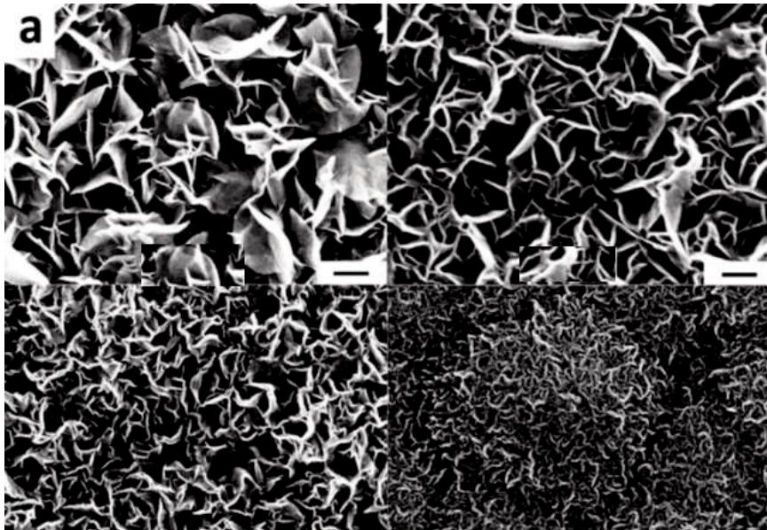
Fig.21 SEM image of Floral-clustered few-layer graphene nanosheet [22]
