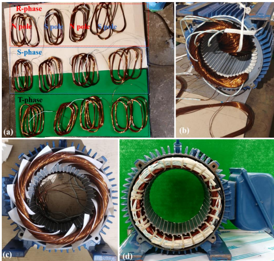
Fig. 5.7. Photographs of fabricated stator for the 1 kW class HTSG. (a) Armature coil modules, (b) armature coil assembly with stator core, (c) insulation in armature ends, and (d) final assembly of the stator
