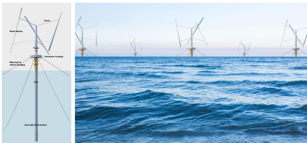
Figure 1.19 Concept illustration of the wind farm with multiple SeaTwirl S2
