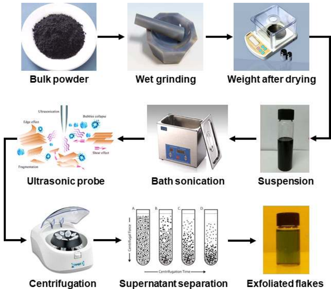
Fig. 6.13 Step by step liquid mechanical exfoliation process used to make suspension of 2D MoS 2 분말s in ethanol
