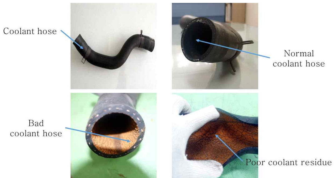
Fig. 42 Comparison of normal and bad coolant hoses
