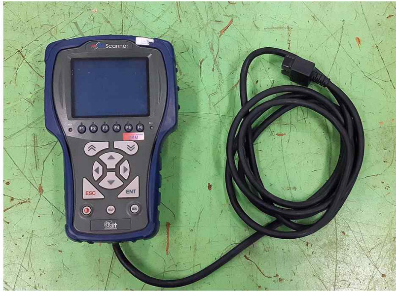
Fig. 2 Hi-DS Scanner with electronic control diagnosis
