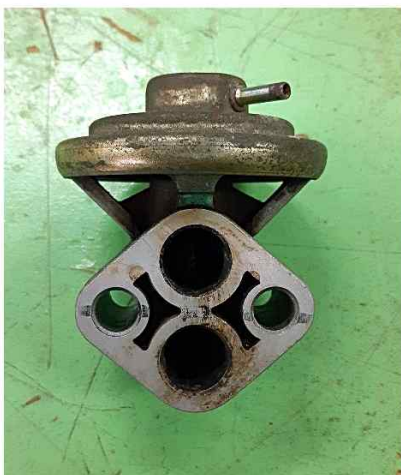
Fig. 33 Operation of the EGR valve
