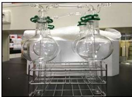
Sampling ammonia gas using impinger (10 mL)
