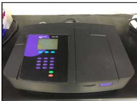
Observing absorbance at 640 nm by UV-Visible spectrophotometer
