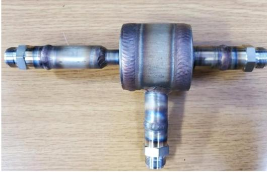
(a) Ejector nozzle size(mm) : 1.0
