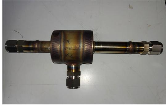
(b) Ejector nozzle size(mm) : 1.8
