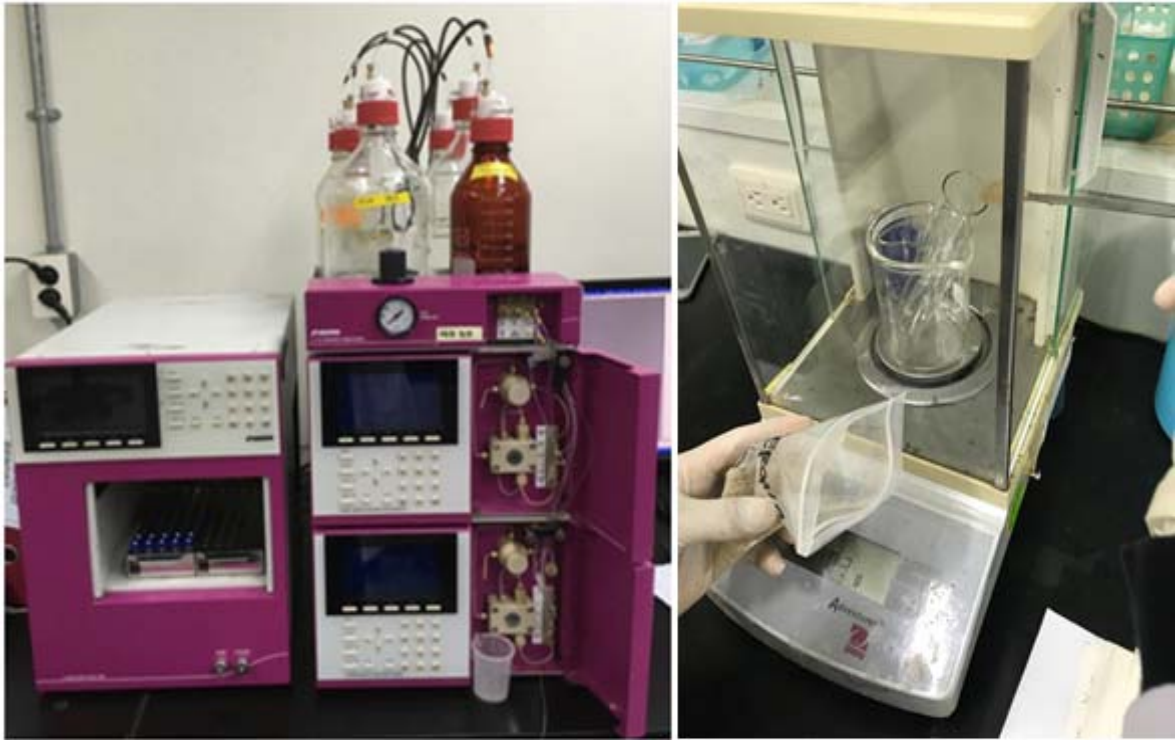
Figure 8. The amino acid (AA) analyzer (SyKam Amino Acid Analyzer S433) (left) and measurement of sample weight for AA analysis (right)
