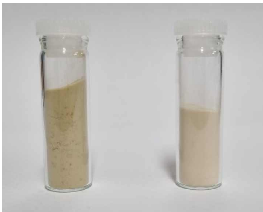
Figure 1. Photo of GA gel and NB gel. (particle sizes of all the gels are sieved 200-400 mesh)
