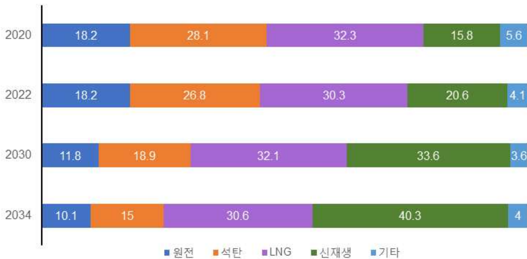
Fig. 1-1 Changes in the ratio of power generation sources according to the 9 th basic plan[1]
