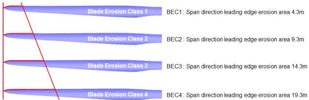
Fig. 4-1 Difference in erosion area according to blade erosion class
