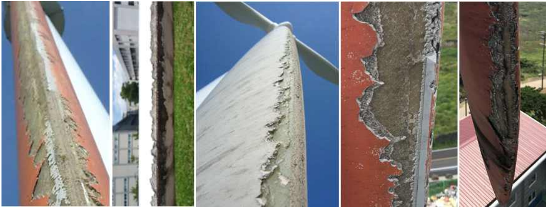
Fig. 2-4 Blade leading edge erosion patterns used in various studies and reports[13, 14, 15]
