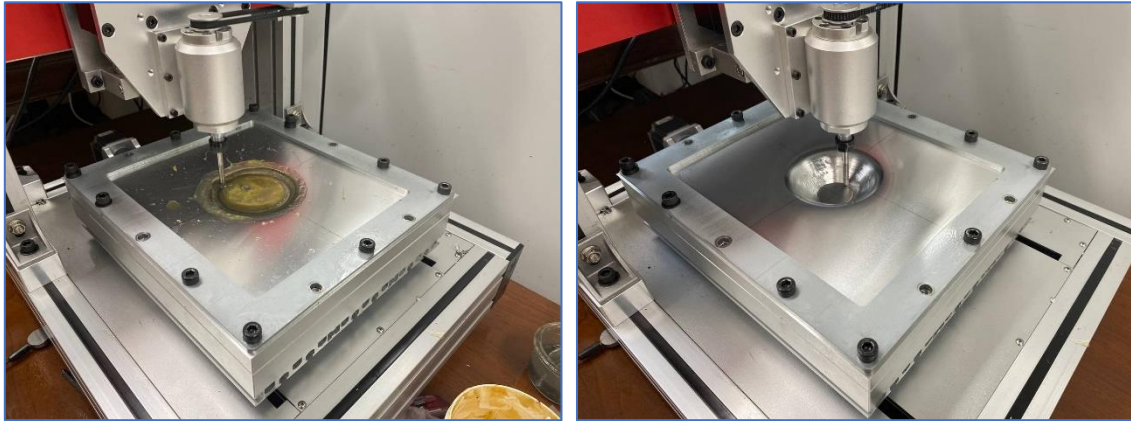
Figure 24. Forming process and last step of SPIF.
