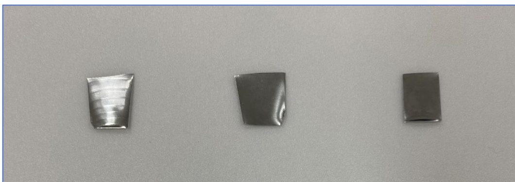
Figure 50. Samples to measure thickness of deformed part of sheet.
