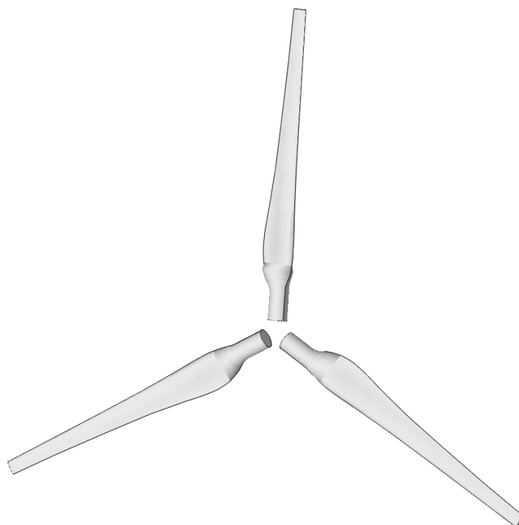
Fig. 37 HAWT REA blades In Q-Blade
