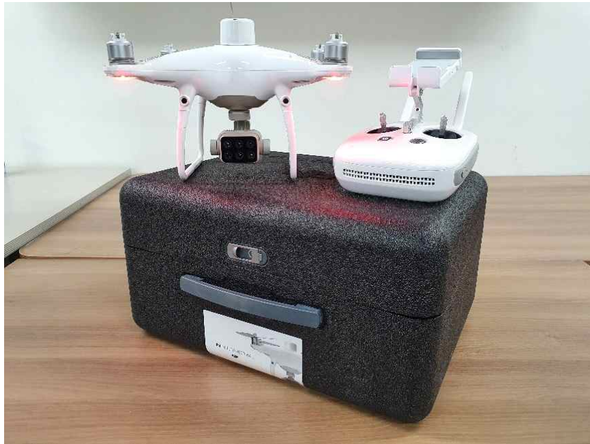
Fig. 4. RGB camera sensor and multispectral sensor mounted Phantom 4 Multispectral.
