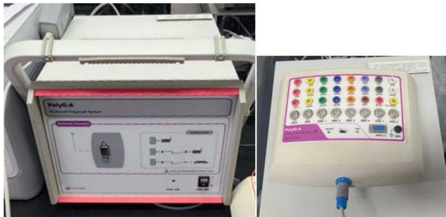
Fig. 4. Equipment of EEG signal measurement (PolyG-A, Laxtha, Korea)
