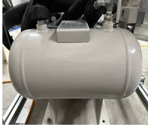
(b) Air receiver tank
