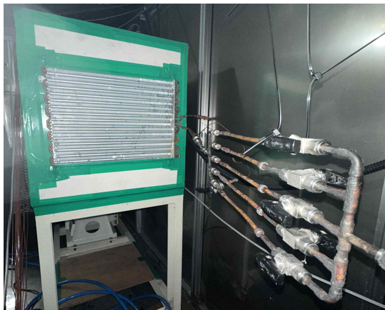
Fig. 16 Measure the cooling effect when nozzles are attached to the evaporator
