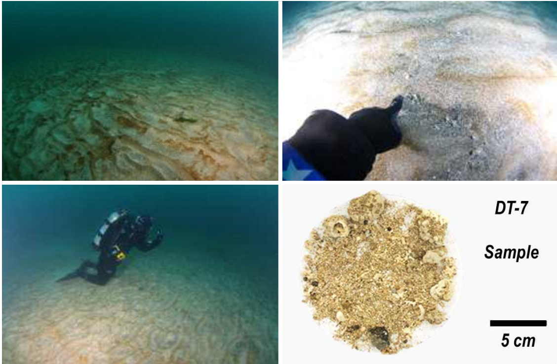
Fig. 3-5. Photos of type B seafloor (DT-7) which is covered by sandy sediments composed of broken particles of rhodoliths and shells. See Table 3-1 for photo location.
