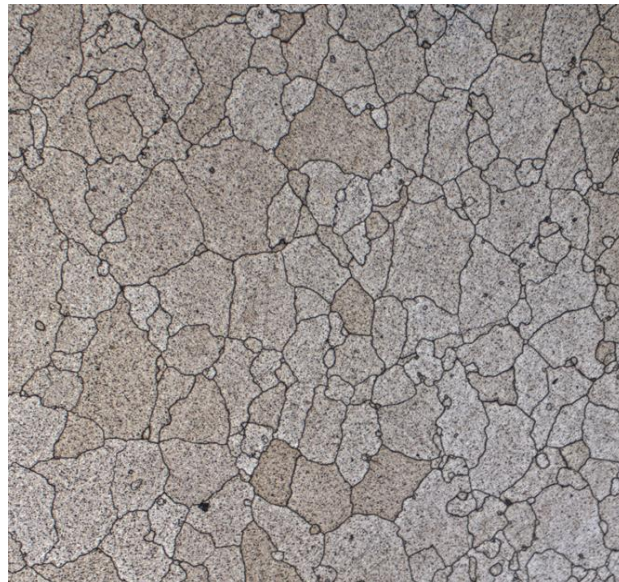
Fig. 2.1 The original metallographic structure of 6061-T6 aluminum alloy
