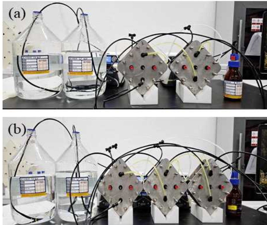
Fig. 42. Photograph of RED of (a) 1 x 2 and (b) 1 x 3 module stack at lab scale
