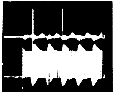
Fig. 3 Photograph of double pulse signal from delay circuit
