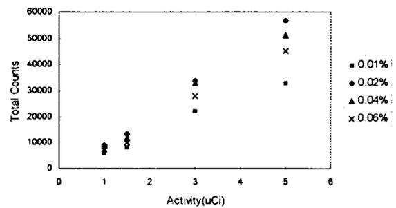
Fig. 8. Proportionality of the total count versus the source activity measured with the sensors having different concentrations of dPOPOP.
