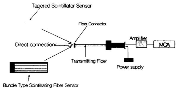
Fig. 2. Experimental setup for the test of the optical sensors
