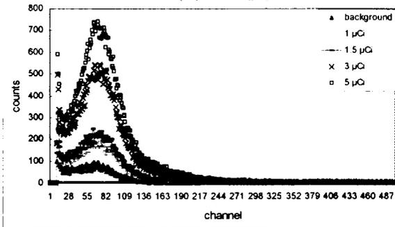
Fig. 5. Pulse-height spectrum measured with the tapered scintillator sensor. PPO and dPOPOP concentrations are 0.1%, 0.02% (mol/ℓ), respectively.
