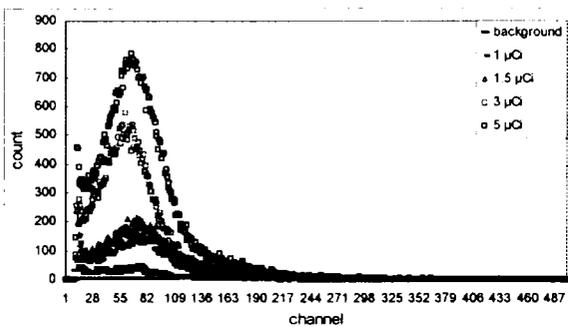
Fig. 7. Pulse-height spectrum measured with the tapered scintillator sensor. bPBD and dPOPOP concentrations are 0.1%, 0.02% (mol/ℓ), respectively.
