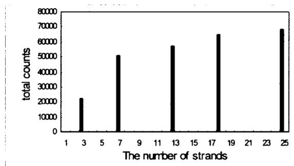
Fig. 4. The total counts measured with sensors having the different number of strands.
