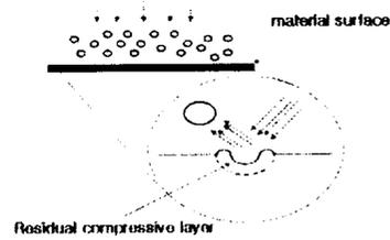
Fig. 4. Schematic diagram of blasting
