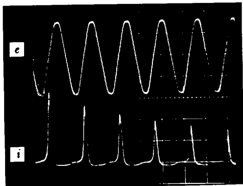
Fig. 6. Measured waveform at θ 1 Voltage 10V/div; Current 20A/div ; Time base 10ms/div.
