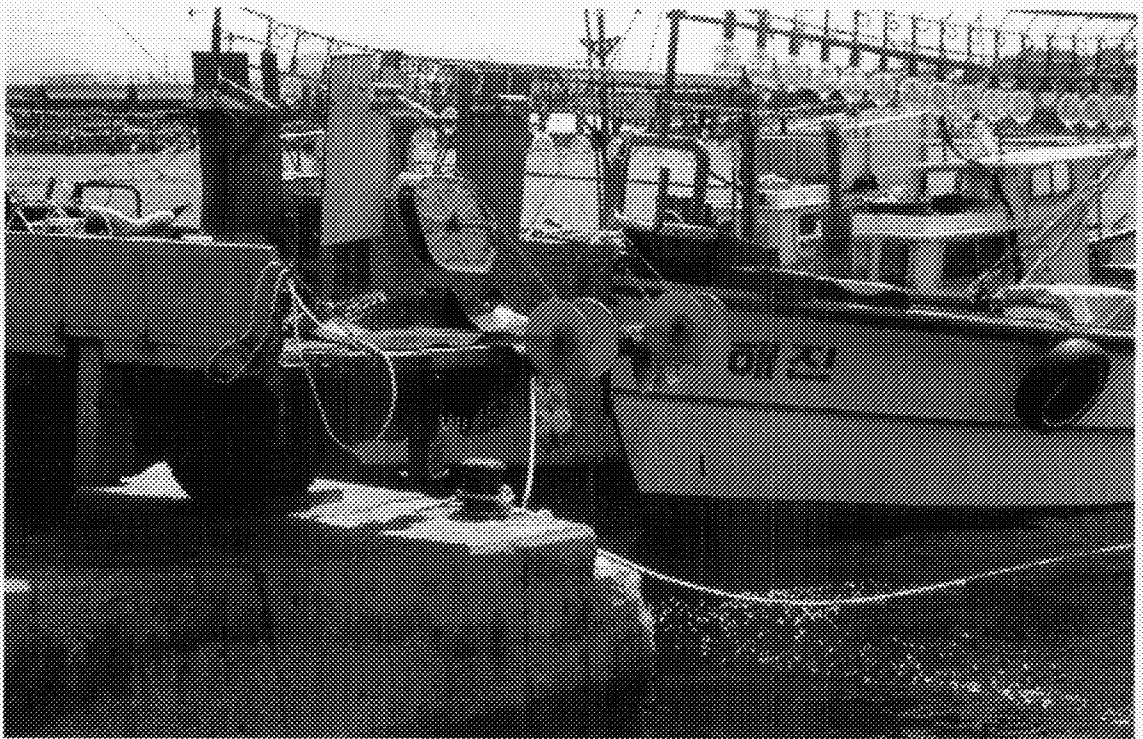
Fig. 2. Photograph of the rotary equipment for revolving a main line of automatic hairtail hand line.
